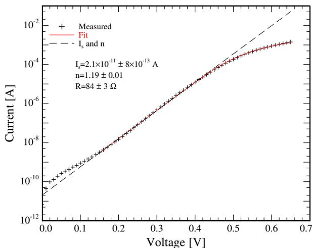
Fig. 5. Current-voltage characteristic of the fabricated photodiode. The photodiode ring has inner radius 3.29 mm and outer radius 4.07 mm yielding an active area of 18 mm<sup>2</sup>.
