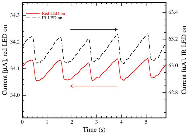
Fig. 7. Photoplethysmograms measured with the developed ring-shaped photodiode.
