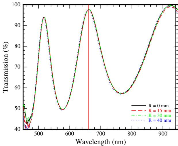
Fig. 4. Transmission of the SiO<sub>2</sub> and SiN interference filter measured with a Filmtek reflectometer. The transmission uniformity across a wafer is seen to be good since there is no significant deviation in transmission between the four plots measured at a radius, R, from the wafer center.
